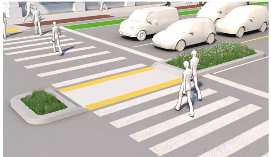
Figure 71: High Visibility Paint, Continental Stripping, Refuge Island / ADA Ramps
