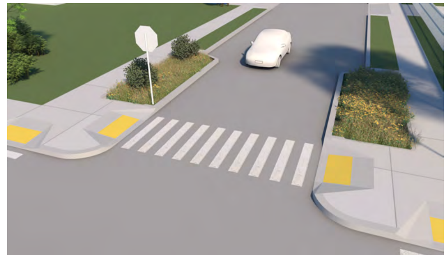
Figure 73: Curb extension with High-visibility paint crosswalk 1
